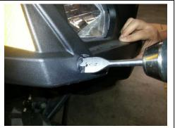
5. To mount the signal, first remove the rubber grommet from the light. Push the grommet into the hole until it is seated correctly into the hole. Feed the wires of the light into the new hole you drilled. Notice the direction on the lens; make sure the "Top" is at the upper point of the light. Plug the red wire from the signal into the positive wire on the harness and the black signal wire into the ground signal wire.
